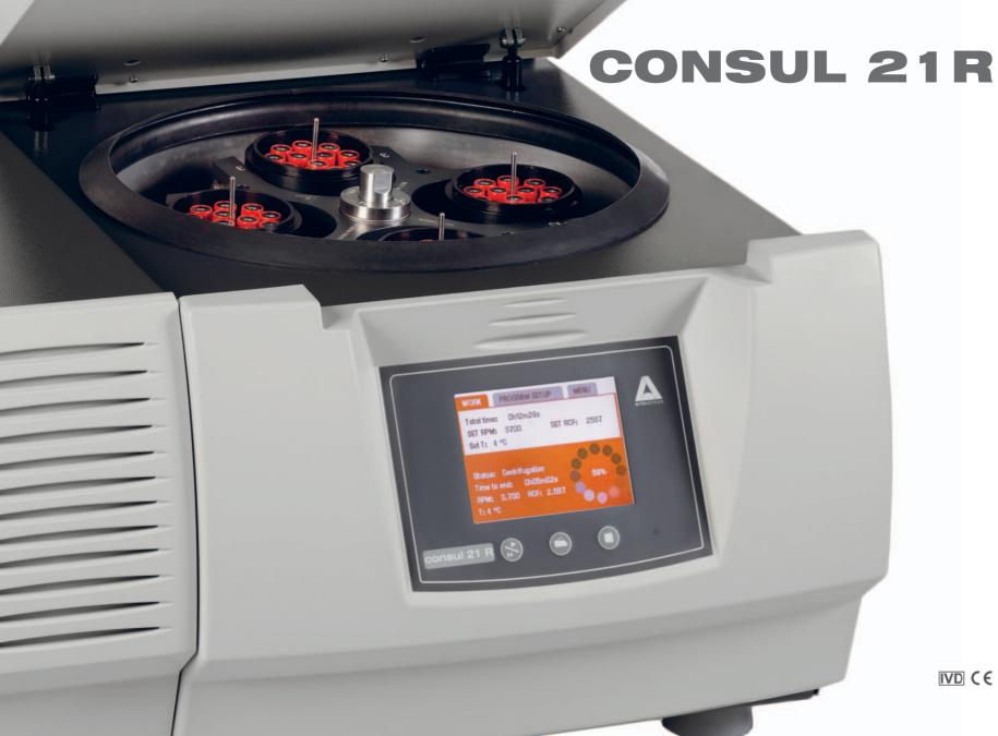
High capacity on a bench top centrifuge which offer to their users several advantages, up to now only available on devices dedicated to research. The TFT touch screen simplifies the parameter selection; main values appear only in one screen as time, RPM, RCF, acceleration and braking.
