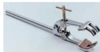
Clamp for flasks or condenser tubes.
