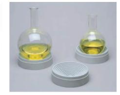
**ROUND BOTTOM FLASK SUPPORT** Made of moulded rubber (E.P.D.M.). Temperature resistance up to 100 °C. Specially designed with stepped surface to support different flask diameters. From 100 ml up to 10 litre capacity. Dimensions: 50 mm high x 160 mm Ø. Part No. 1000863
