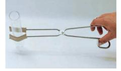
TONGS FOR FLASKS AND TUBESElectro-bright finished AISI 304 stainless steel.For diameters from 15 to 60 mm.Tong tips covered with stabilized glass fibre.Part No. 1028130Part No. 1028140Total length 300 mm.Part No. 1028140Total length 400 mm.
