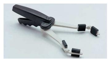
BEAKER TONGS "PROTECVAS" Clamps beakers up to 2000 ml. With a span from 50 to 120 mm Ø. Jaws protected with rubber pads. Total length 300 mm. Part No. 7000532
