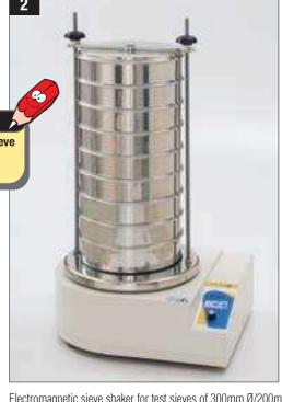
Electromagnetic sieve shaker for test sieves of 300mm.Ø/200mm.Ø
